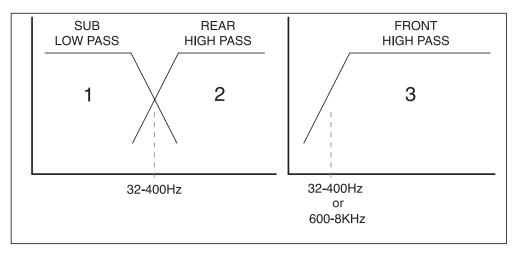
3 way system with front and rear fader
