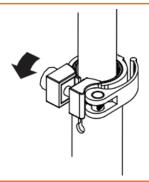
To unfold the scooter, pull the release lever downwards toward the deck while pulling upwards on the steering column.
