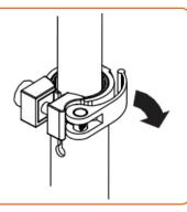
The tension of the guick release clamping mechanism can be adjusted by tightening or loosening the Allen bolt. Be careful not to over tighten. You should always be able to open and close the quick-release lever by hand and the T-tube should telescope freely with the quickrelease open.
