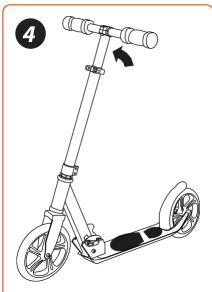
Release the lever and continue to unfold the steering column upward. grip the handlebars and place one foot on the deck. Pull the handlebars up until the latch engages. Make sure the locking mechanism is secure in the open position before riding.
