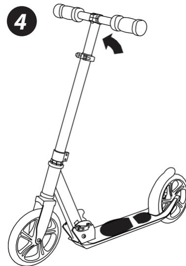
Release the lever and continue to unfold the steering column upward. Grip the handlebars and place one foot on the deck. Pull the handlebars up until the latch engages. Make sure the locking mechanism is secure in the open position before riding.
