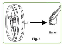
Press the button on the wheel holder to assemble the rear wheel as Fig. 3.
