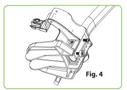
Remove the screws and Plastic piece as Fig. 4. Take out the fixed steel piece from instruction PE bag, then going the screws through the holes and keep the "up" toward front as Fig. 5.
