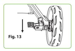
Push on the brake pedal to stop the rear wheel and pull off to release as Fig. 13.
