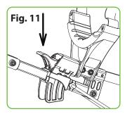
Press the button and adjust the slide lock to required handle height as Fig. 11.
