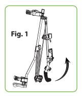
Lift the handle to level position as Fig. 1
