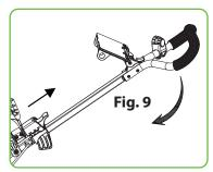
Move the slide lock up to release the handle as Fig. 9.
