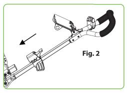
Move the slide lock downside and lock to upper bracket as Fig. 2
