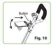
Press button to adjust the scorecard holder to required height position Fig. 10.
