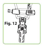
The buckle can move from the front to the back as Fig. 10. The wheel can swivel when the buckle is on the "A" position as Fig.11, and the wheel can go straight line when the buckle is on the "B" position as Fig. 12.
