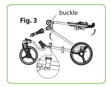
Open the fixing strap and buckle to unfold the cart as Fig. 3.
