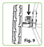
Push down brake pedal to stop the rear wheel and raise up to release the rear wheel as Fig. 9.
