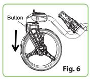
Press the button to take off the front wheel as Fig. 6.
