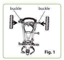
Assembly rear wheel sets insert the wheel holes then press the buckle towards down as Fig. 1.
