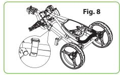
Release the buckle, fold Fix the velcro strap around the upper the upper frame and the and lower frame as shown Fig. 8.
