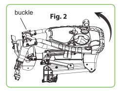
Release the handle buckle to fully extend the handle frame then lock the locking buckle as Fig. 2.
