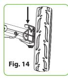
Using the brake Press the brake pedal to stop and press again to release as Fig. 14.
