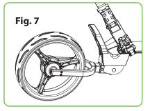
Remove the M6\*40 screw and M6 nut from the front wheel fork as Fig. 6, then assemble the front wheel on the steel piece of lower bag bracket and fixed it by screw and nut, completely assembly as Fig. 7.
