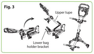
Hold the upper tupe and lower bracket to open the frame as Fig. 3
