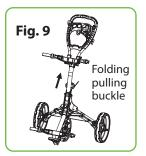
Pull the folding pulling buckle and press the handle to fold the trolley as Fig. 9 & 10.
