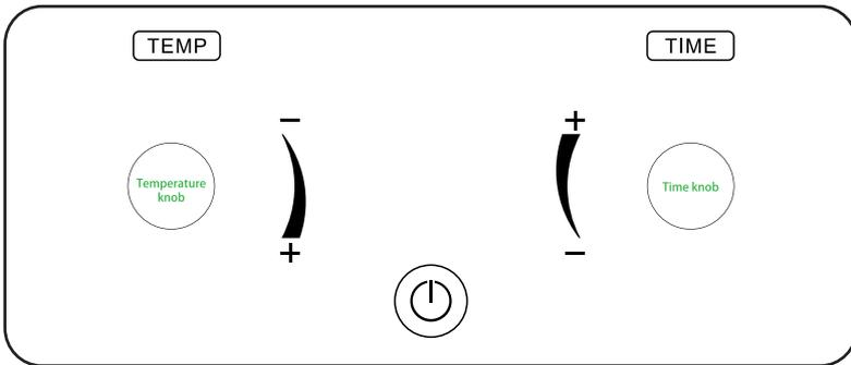
1. Plug dehydrator into wall outlet, the screen light up and there is a beep sound at the beginning when it starts up. After one second, the product enter to the standby mode. Then, the temperament shows "000", the time shows "00", the other icon will be off.
