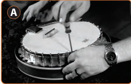
To tighten it up, first take off most of the thumb screws which hold the resonator to the flange so you can access all of the lugs that tighten the head.
