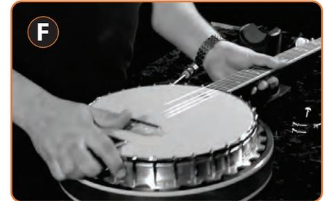
Replace the resonator to the banjo assembly and tighten back all the thumb screws.
