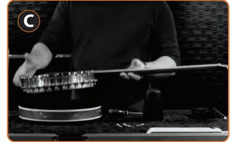
Remove the banjo assembly from the resonator and set that aside.
