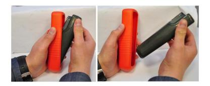
2. Battery compartment is located in the rear of the gray plastic unit.
