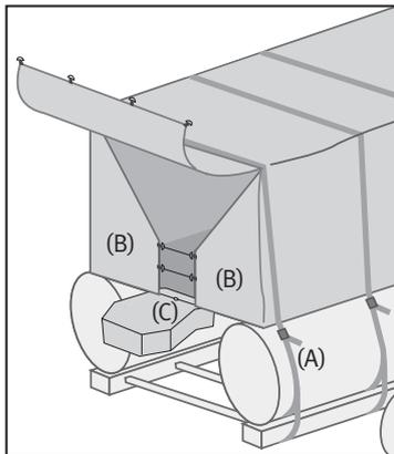
5. To secure the transom flap, first locate the adjustable cover side panels (B) and wrap them towards the center of the boat. Secure them in place by hooking the hem elastic cord hooks (C) together. Cinch the D-rings on the adjustable side panels together using the two provided hooked elastic cords.
