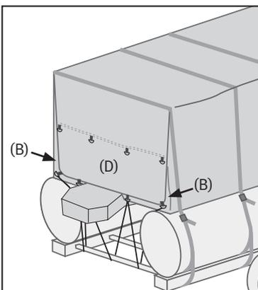
Fold the transom flap (D) over the side panels (B) and adjust the transom flap (D) to determine which row of D-rings on the transom flap allows you to best cover the stern of your boat. When using the top row of D-rings, tuck excess transom flap under. Secure by tying the provided rope to an end D-ring then weaving the rope from the D-ring to the trailer
