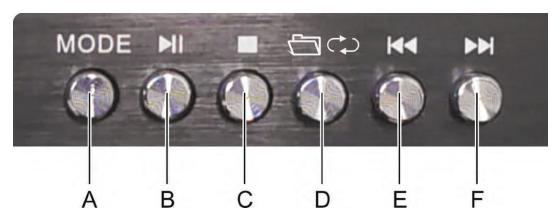
A. MODE BUTTON: Press this button to select one from play mode with USB/SD mode, FM mode and Wireless BT mode, automatically set in USB/SD mode after turning on the unit, automatically play mp3 files after inserting a USB flash driver or SD card.
