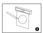
Cut the drywall. Note:Always allow at least one-half inch between a wall stud and the speaker cutout or the locking tabs will not be able to swivel into place.
