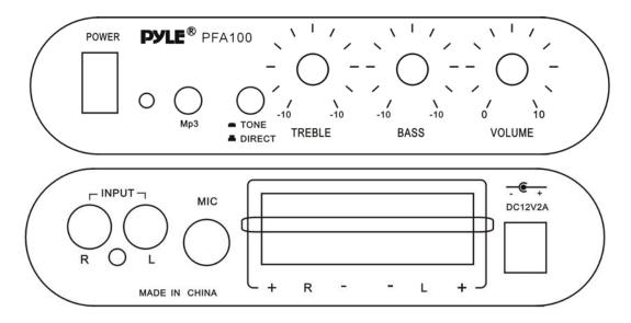
Front Inputs: 3.5mm (1/8") Rear Outputs: Speaker, RCA L/R, ¼" Mic
