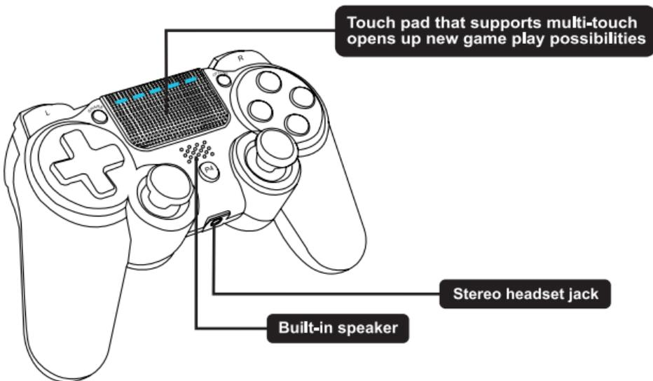
**There are several built-in output connection ports in the controller:** 3.5mm headset jack, Micro-USB charging port, extension port and built-in speaker. Among them, the 3.5mm stereo headset jack can connect headset and microphone, allowing Users to receive and transmit audio at the same time.
