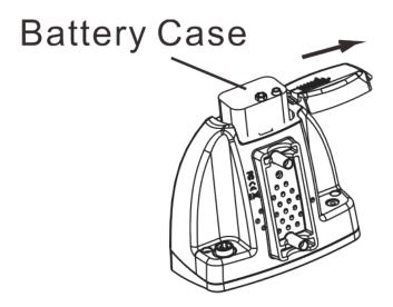
Once the batteries are inserted correctly, replace the battery cover. Don't mix the new and old batteries. If you don't use the detector for a long time, please remove the batteries from the battery box.
