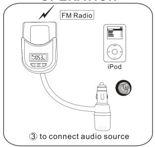
Adjust the frequency of car FM radio to the same frequency as transmitter for receicing signals.
