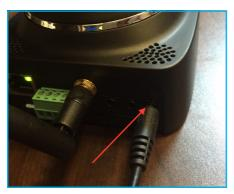
**3.** Reset the camera using a pin - Hold in the reset pin for 10 - 12 seconds until you hear an audible chirp. Wait again 1 - 2 min for the camera to reset and run through the full range of pan and tilt
