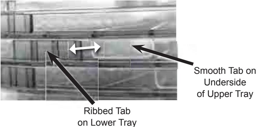
For round trays, to change the spacing between trays, it is necessary to identify the stacking tabs. The tabs with the three reinforcing ribs shown above are on the lower tray, and the smooth tab is part of the top tray in this photo. Note that they are next to each other as indicated by the white arrow. This is the alignment for thinner foods. This is also the best position for storage of the appliance since the total stack height is minimized.
