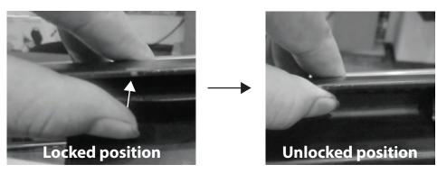
Please lift the glass lid along the slot to the top baffle position then push and close the glass lid lock to the bottom housing. Machine may be damaged if its not lifted up glass lid to the baffle.
