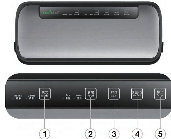
1. **"Mode" button:** it has two setting mode (Normal and Gentle). The default mode is Normal. When the food is crumbly, press the button then the vacuum mode is changed to Gentle. You can manually control the degree of vacuum by pressing "Seal button" at any time, the food will be sealed automatically. (**Note: if the power is interrupted, this setting will return to a preset standard mode**).
