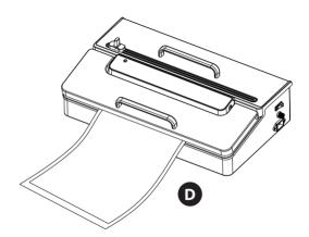
3. Press the cover down with a little pressure to make the sealing gaskets better matched closer, the next step is same as vacuum or seal process.
