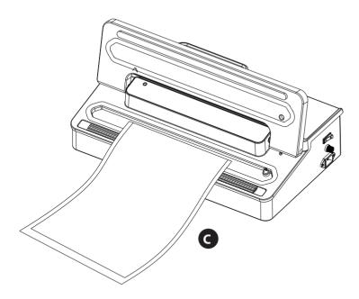
2. Put the opening of the bag in the vacuum chamber. Make sure the bag does not cover the vacuum nozzle
