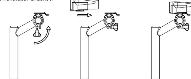
Releasing the MP3 loudspeaker player from the handlebar bracket.
