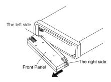
3. For safekeeping, store the front panel in the supplied protective case immediately after being removed.
