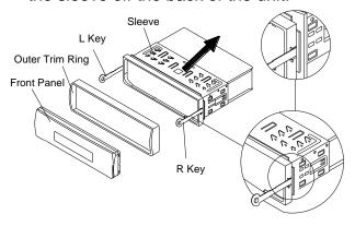
6. Mount the sleeve by inserting the sleeve into the opening of the dashboard and bend open the tabs located around the sleeve with a screwdriver. Not all tabs will be able to make contact, so examine which ones will be most effective. Bending open the appropriate tabs behind the dashboard to secure the sleeve in place.
