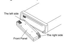
2. When the two sides fixed into place, push the front panel into main unit.
