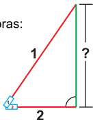
Indirect measurement determining a distance using 2 measurements
