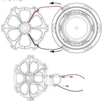
**STEP 3.**Put the grill back to the speaker and fasten the screws.
