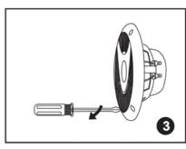
Screw down each of the four Phillips head screws.The locking tabs will swivel into place and secure the unit to the rear surface of the drywall. Put in the strips of adhesive to secure the grille.
