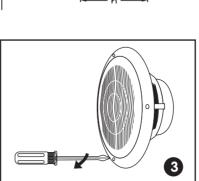
Screw down each of the four Phillips head screws.The locking tabs will swivel into place and secure the unit to the rear surface of the drywall. Put in the strips of adhesive to secure the grille.
