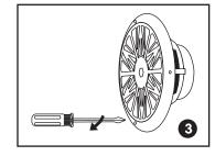
Screw down each of the four Phillips head screws.
