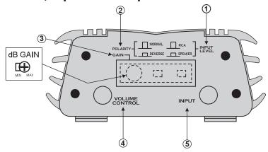
The switches and gain settings are located behind a watertight plug, which also lights up when the amplifier is on. Be sure to replace the plug when finished with adjustments.
