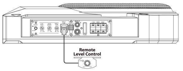
Instal the remote control securely under the dash or in a similar location where using it will not distract the driver.
