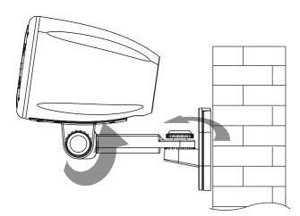
The front bracket can be rotated up and down, and the rear support can be rotated around.
