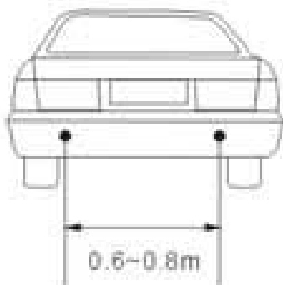
Install two sensor
