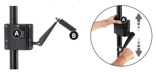
To crank up or down, firstly press the button **A**, and then shake the crank handle **B**. When cranking up or down, you need to keep pressing the button **A**. After cranking to the desired height, let go of button **A** and then tighten the clutch.
