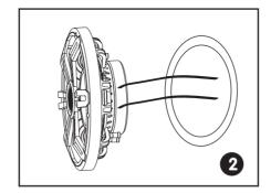
Connect the speaker wires to the speaker.
