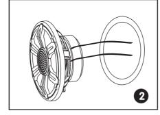
Connect the speaker wires to the speaker.
