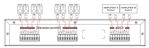
4-Way Dual-Source, High-Power, Autoformer-Based, Impedance-Matching Speaker Selector with Zone Volume Controls
