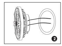
Connect the speaker wires to the speaker.
