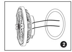
Connect the speaker wires to the speaker.
