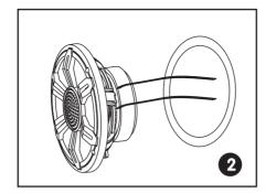
Connect the speaker wires to the speaker.
