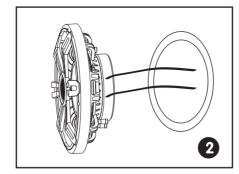
Connect the speaker wires to the speaker.
