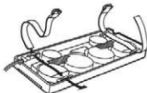
Fasten the speaker unit to the sunvisor with the belt
