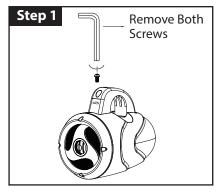
Remove the two screws from the bracket to separate the speaker pod and the bracket.
