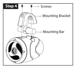
Screw the two screws evenly, until snug. Once the position is verified, tighten the screws another half-turn. **DO NOT OVERTIGHTEN!**
