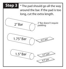
Remove the backing off the pad and wrap it around the bar.
