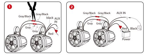
Step 8: Connected two speakers by RGB connect wire, see the drawing in below (See Illustration 3)
