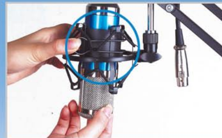
7 Slide Your Microphone into the Shelf Clip Ring
