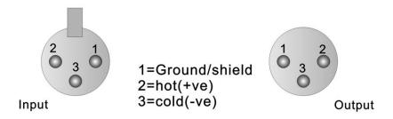
For unbalanced use pin 1 and pin 2 have to bridged
