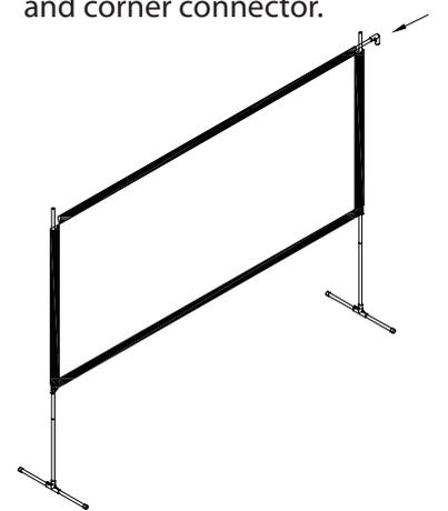
4. Insert the corner connector into the vertical poles on both sides
