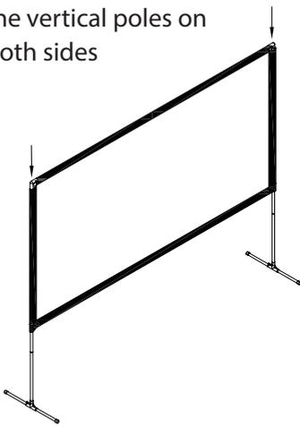
5. Push the vertical rod to both sides to make the screen equal width up and down.
