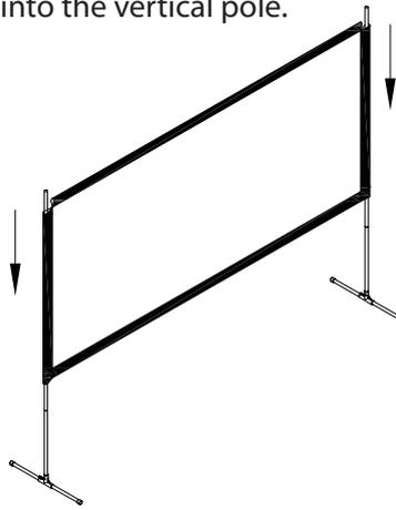
3. Insert the upper transverse pole and corner connector.
