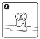
Use the metal clip to attach the screen on the top bar then use the zip tie to go through the hole and fix the screen on the top bar.
