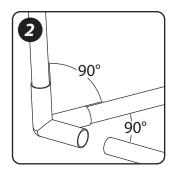
Insert the metal frame into the 3 Way Pipe Fittings. The tube must be fully inserted into the 3 Way Pipe Fittings as much as possible.
