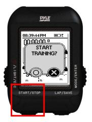
3. During the training, you can press the Down/LAP button to create a new lap Or press ENTER to switch between the four workout pages.
