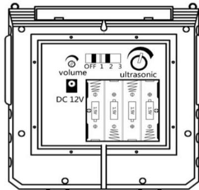
Mode 1 – Audible Repellant - uses a series of seven different recorded sounds (GUN SHOT / SIREN 1 / BOAR SQUEAL / SIREN 2 / BANGING SOUNDS / SIREN 3 / DOG BARKING). The repeller will cycle through these sounds, preventing animals from getting used to any one sound and increasing its effectiveness. Adjust the loudness as needed.
