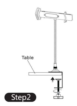
Clip on the table and tighten it by screwing
